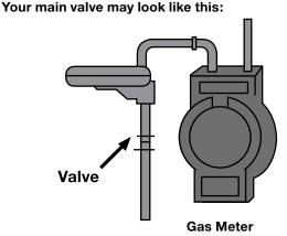
To turn gas off, give the valve a quarter turn in either direction. When the lever crosses the direction of the pipe (see below) the gas is off.
